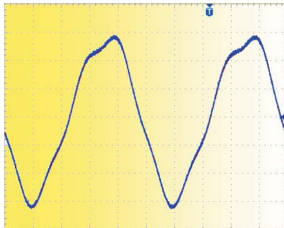
90A peak current / 50Hz with 3rd harmonic distortion Timebase: 4.0ms per division Channel 1: Class 0.2 current transformer Channel 2: LFR03/3, 100mV/A, Phase error <math>< 0.85^\circ</math> at 50Hz
